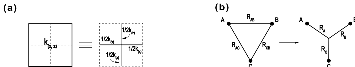
Figure 4. (a) We represent each cell with a cross of unequal resistors (i.e., 1/k_x \neq 1/k_z ). (b) Star-triangle transformation yields an equivalent circuit for three nodes joined by three resistors.
